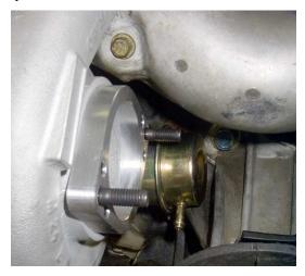
The right side turbo can be installed without modifying the motor mount support, if you are installing the turbos with the engine removed from the car. You must first install the turbocharger, then reinstall the motor mount support after the turbo is in place.
