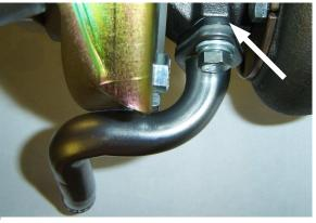
Install the supplied oil drain spacer as shown on the left side oil return tube to clear the compressor housing. Slot both oil tubes at the bolt holes to fit the newer ball bearing format bolt holes. Use stock 300ZX drain gaskets and slot them, if not supplied.
