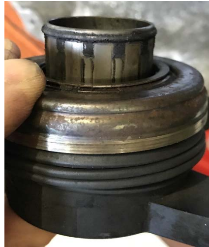
Clutch dust built up along the 12 axial slots.
