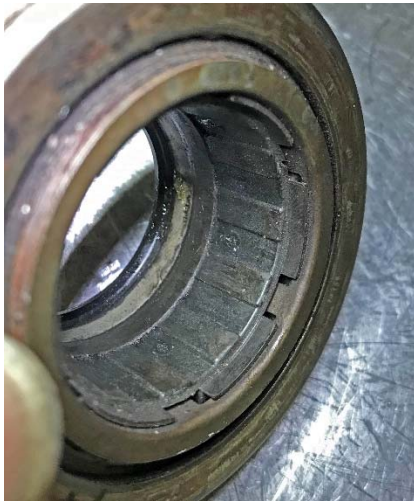
Axial slots directly exposing the seal to clutch dust.
